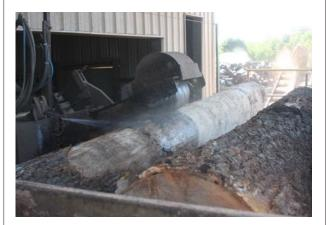
At the mill, the bark is first removed from the log. All bark, saw dust and other non-usable wood fiber is collected and used for other purposes, like heating the facility or manufacturing wood pellets or mulch.
