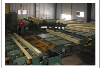
The square logs are next cut into wood slabs at a predetermined thickness, maximizing the usable lumber. The slab edges are then trued and trimmed square, creating what we typically call a lumber board.
