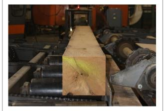
For sawn or sliced material, the rounded edges are then removed to produce a square log called a cant.
