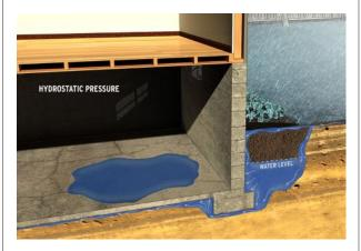
Hydrostatic pressure can occur only when exterior water levels are above the bottom of the slab. As such, it only develops in "below-grade" applications. Moisture issues related to hydrostatic pressure are avoided by using adequate drainage systems and/or waterproofing membranes around the foundation of the structure.
