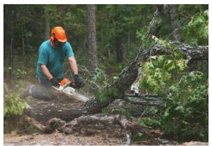
Next, the log is rough cut to the desired length. Maximum lengths are maintained whenever possible. All branches are cut (limbed) from the log. The logs are then removed from the forest, loaded onto logging trucks, and delivered to the mill yard.
