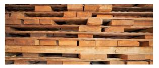
After sorting, boards are stacked to facilitate air movement and begin the air-drying process. This is accomplished by placing small, thin boards called "stickers" between each stacked layer of wood. This maximizes air movement, which helps to bring the moisture content of the lumber into equilibrium with its surrounding environment. The temperature, humidity and airflow will influence the time needed to reduce moisture content of the wood. The goal is generally to reach 18-30% moisture content.
